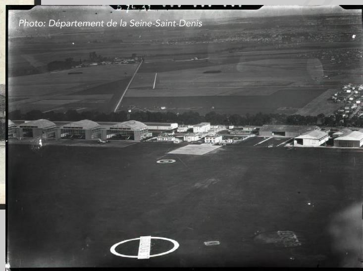
➤ Photo: First aerial photo taken of le Bourget Airport near Paris in 1921, showing the hangars and the “LE BOURGET” target sign in the middle of the airfield to help pilots locate the correct landing field among the many other fields around.
