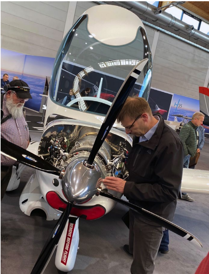
Small 140 HP Turbine on a Bristell aircraft
