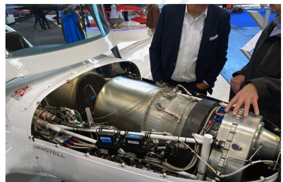
Small 140 HP Turbine on a Bristell aircraft, showing how small the turbine is.
